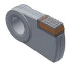
Hammer type crushers are characteristic of advanced structure, excellent performances, big crushing rate. They have become crushing equipment for cement, mining and sand processing industries. The too short lifetime of hammers and quick wear of the metals has become an outstanding problem for such equipment.
