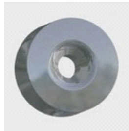
Tungsten carbide pressure cylinders as sintered
